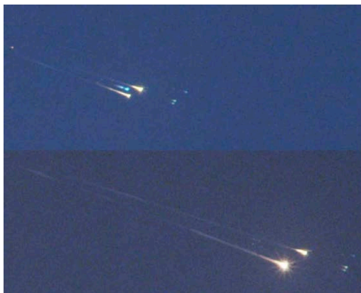
Figure 6. Fragmentation of WT1190F. These Red EPIC single frames were taken just after the main fragmentation event (top) and at peak brightness (bottom).
